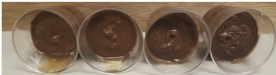
Figure 8.5 Chocolate spread stabilized using 0, 4, 10, 15 wt% oleogelator (of the oil phase) after 21 days in 40 °C incubator.
